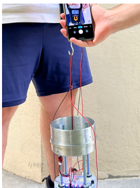
Fig. 4.34: Connector 3 test (drogue).
