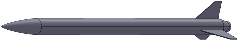
Fig. 2.9: Simplified model for CFD analysis.
